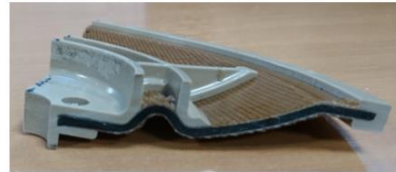
Sensors embedded in battery casing lid thanks to nano-ink printed electronics and overmould process of thermoplastic composite for lightweight property
