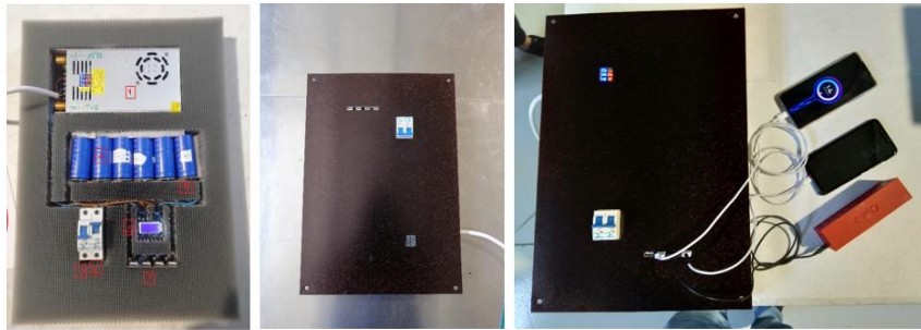
Demonstrator panel with integration of Pleione's supercapacitor module to the final supercapacitor Power Bank
