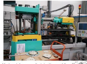
Horizontal composite injection molding machine
