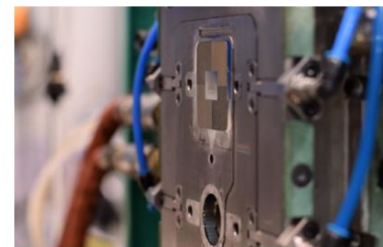
Injection mold with nanostructured surface
